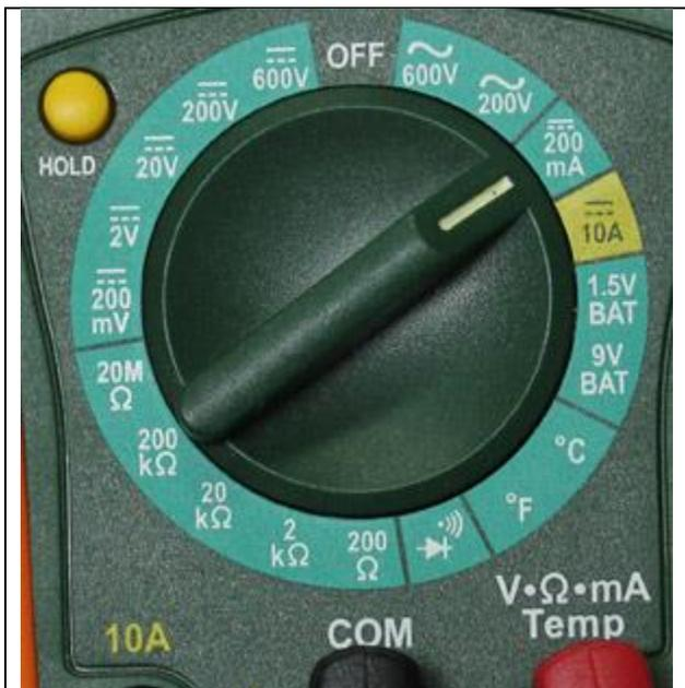
Figure 4 manual meter set to measure current (200 milliamps maximum)
