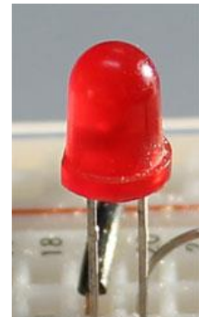
Figure 2. Red LED inserted into breadboard
