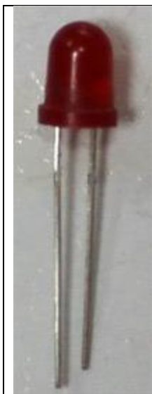
Figure 4. Red LED. The short wire is the cathode and long wire is the anode
