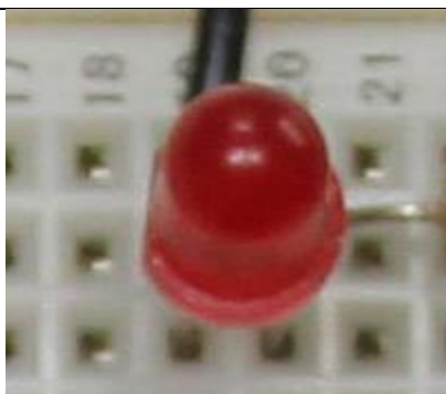
Figure 5. Red LED inserted in the breadboard. The flat side of the LED on the left marks the side with the cathode wire. The cathode must be connected to the negative side of the battery.
