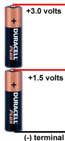
Figure 9 two batteries in series
