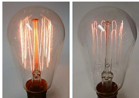
Figure 6 – left -evacuated bulb, right - filled with inert gas
