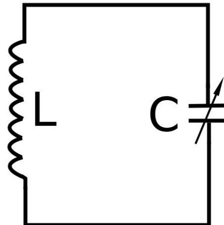
*Figure 2 Schematic of an LC circuit*
