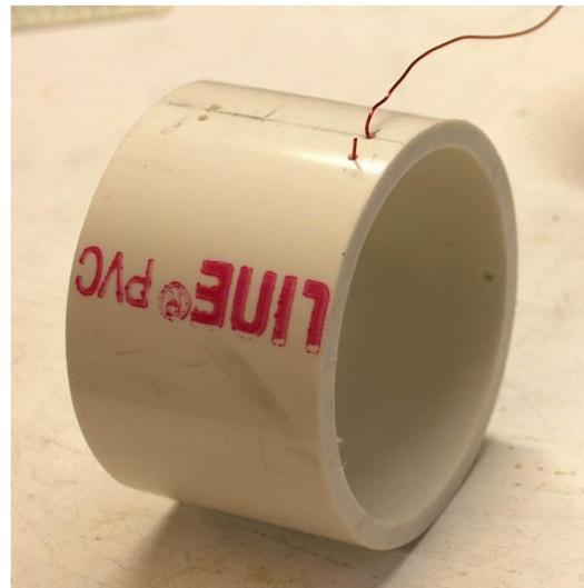
*Figure 4 preparing the coil form for winding*
