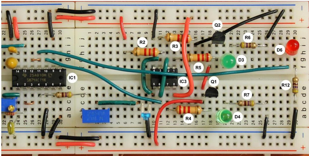
The voltage comparator IC3 should already be inserted on the board with its notch on the right side. Pins 1 and 8 are inserted into row 13 of the board and pins 4 and 5 in row 10.
