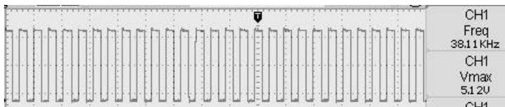
The image above is a copy of my oscilloscope screen after I adjusted R8 to obtain a pulse rate of 38 kHz. Notice that on the right the frequency is displayed as 38.11 kHz. Well, this is not exactly 38 kHz, but it is close enough.
