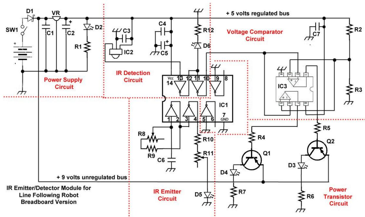
The module schematic above is divided into five circuits. The voltage regulator (VR) of the Power Supply Circuit provides five volt regulated power to IC1, IC2 and IC3. Direct supply of power from the nine volt battery to IC1 and IC2 is not possible because their maximum voltages allowed are 6.0 and 5.5 volts respectively.
