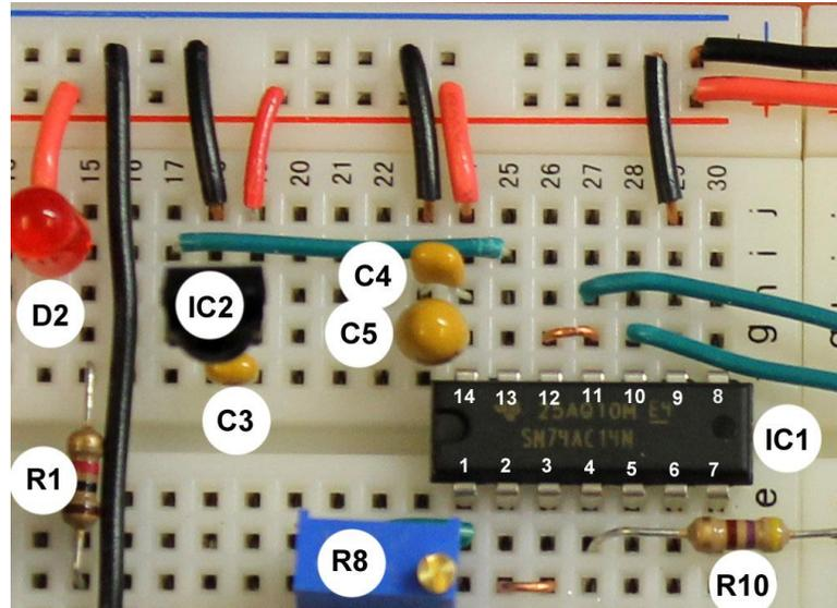
3. Prepare a black jumper wire and connect one end to the top negative power bus and the other end to row 18. This connects the middle pin of IC2 to the negative power supply as needed.
