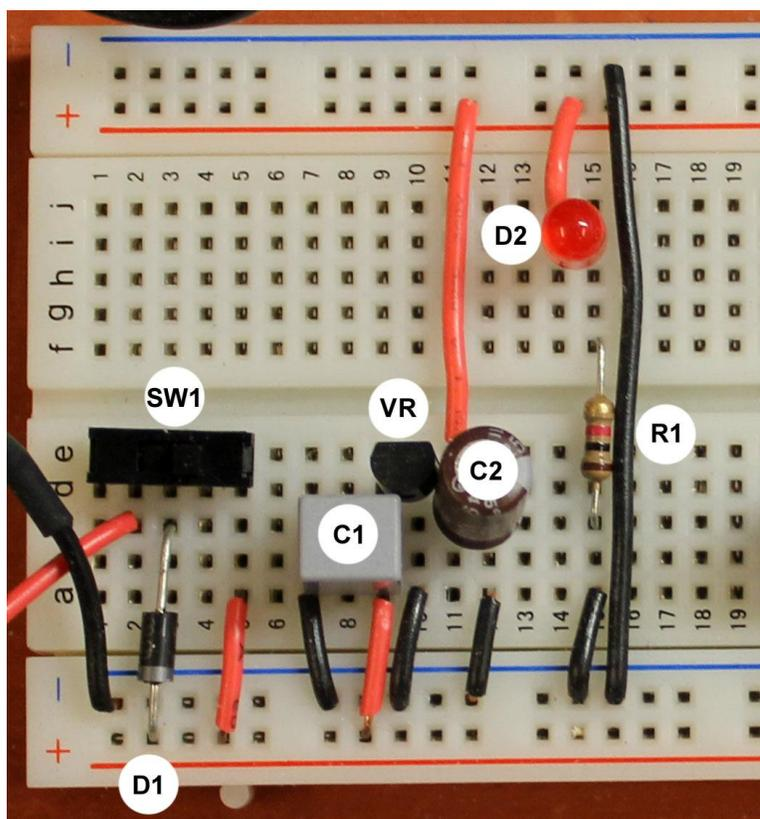
3. The red wire just to the right of D1 is not needed, please disregard. Insert film capacitor C1 (1.0  $\mu$ F, 63 volts) with one pin in row 7 of the board and the other pin in row 9.
