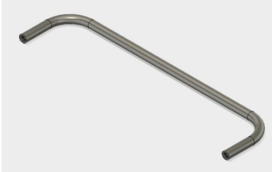
You will be creating a drawer handle like the one illustrated to the left. The procedure requires the drawing of two sketches: 1) a sketch of the path for the sweep and 2) a sketch of the cross section of the handle, which is a circle. The image below provides the dimensions of the handle. Note that the ends of the handle have threaded holes to accommodate screws.
