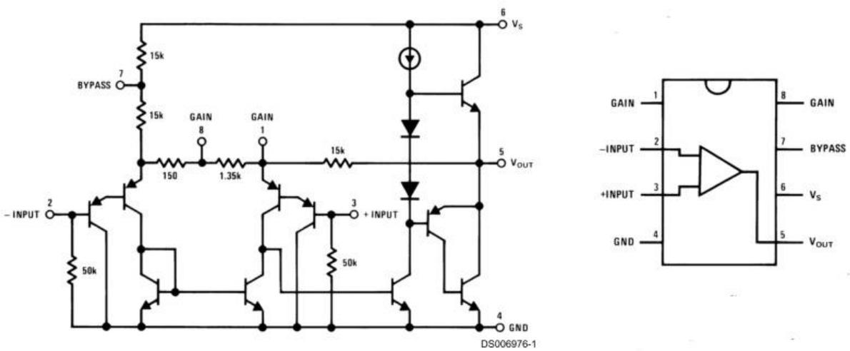
Figure 4 schematic of IC LM386 - audio amp IC chip
