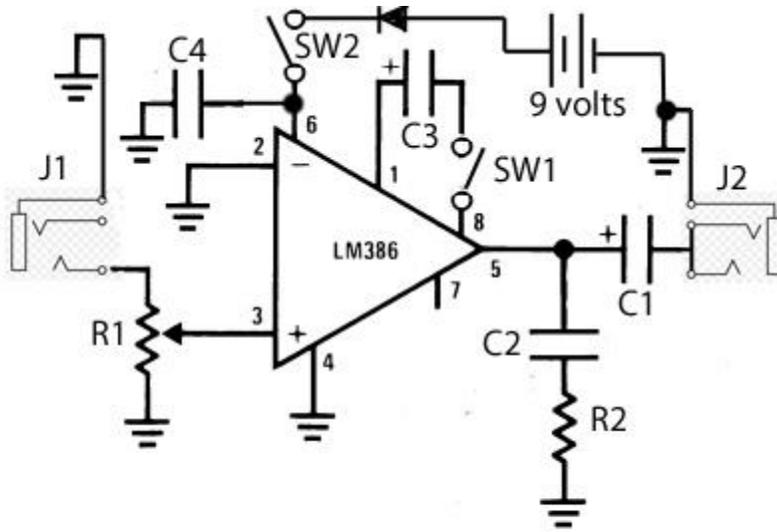
Figure 3 audio amplifier schematic
